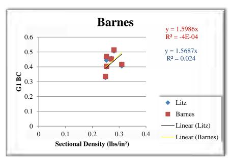
Figure 1: G1 BCs from Barnes and Litz plotted vs. sectional density, along with best-fit lines.
